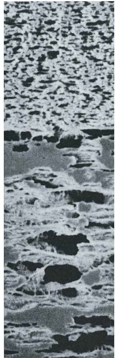
Picture of PTFE membrane cross section taken by using electron microscopy
