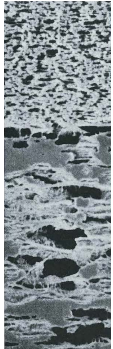
Photograph of PTFE membrane section by Electron Microscope
