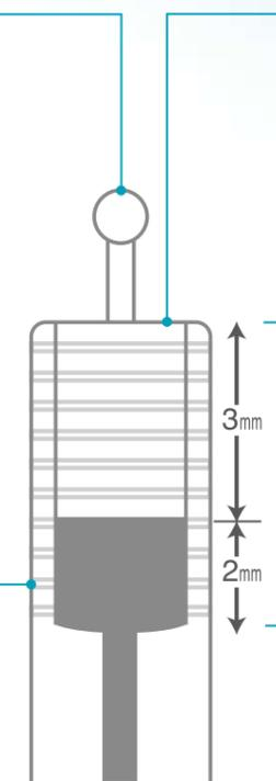
Gradation indication serves as a guide for the protruding length. (White 3mm/Black 2mm)
